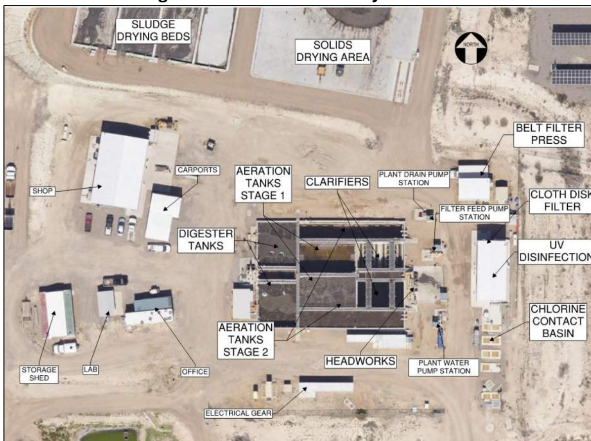
Figure 2-2 Treatment Facility Site Plan
